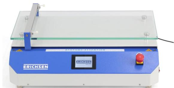
The microprocessor-controlled, precisely graded step motor drive engineering guarantees an extremely uniform accomplishment as well as an excellent repeatability of all processes set.
