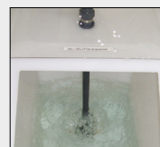
Air agitation of salt solution ACC96
