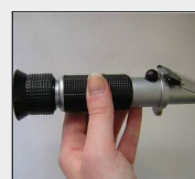
Hand-held salinity refractometer ACC100
